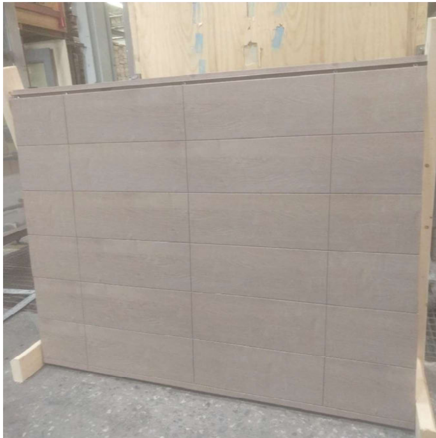
Photo No. 1 View of Test Specimen Prior to Impacts with Stud Spacing Marked
